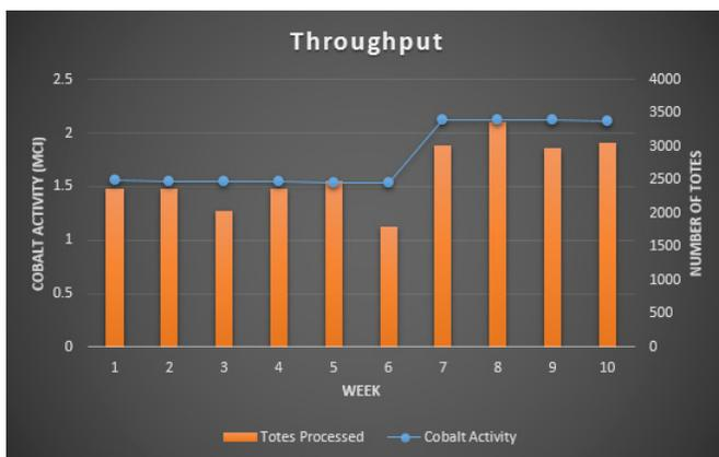
Historically, irradiator operators can easily extract how many totes were processed over a given period. This information is obtained by counting the cycles throughout this period. In the example above, throughput goes up when additional cobalt is added.
